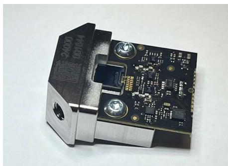
The world's smallest density sensor for liquids with laboratory accuracy! The "core version", without housing, allows the use in apparatus engineering in the smallest installation space. Thus, there is no need to go to the laboratory for reliable measurements. Thanks to a sub-millimeter measuring channel, the properties and quality of a liquid can be precisely monitored even in confined spaces.
